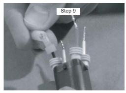
Insert a wire of the Bosch Universal Oxygen Sensor into the male end of the Posi-Lock connector. Keeping slight pressure on the wire, hand tighten the male end into the Posi-Lock barrel. Repeat for the remaining wires of the Bosch Universal Oxygen Sensor, and insert wires of the OE Sensor connector into the male ends of the Posi-Lock connectors.
