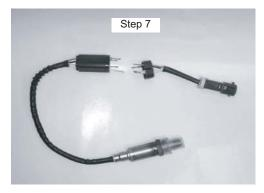
Utilizing "Wire Color Reference Table", match the wires of the OE Sensor connector (column A) to the wires of Bosch Universal Oxygen Sensor (column B). Install the Connector Cap over the wires of the OE Sensor connector. Install the Connector Body over the wires of the Bosch Universal Oxygen Sensor.
