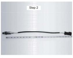
If there are special clips or grommets attached to the OE Sensor, proceed to Step 3. Otherwise, if the length from the hex/flange face to end of OE Sensor connector housing is less than 29 1/2", proceed to Step 4, otherwise, proceed to Step 5.
