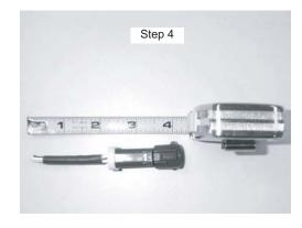
Cut the wiring of OE Sensor 4" from end of connector as illustrated. Lay the Bosch Universal Oxygen Sensor beside the OE Sensor and cut the Bosch Universal Oxygen Sensor wiring to the length of the OE Sensor. Proceed to Step 6.
