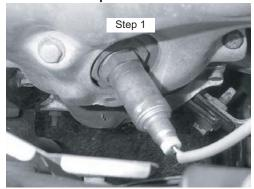
Remove the OE Sensor from vehicle. This is a sample installation location. Oxygen sensors can be located in a manifold or exhaust pipe.
