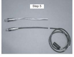
Lay the OE Sensor beside the Bosch Universal Oxygen Sensor and cut the OE Sensor wires to the same length as the Bosch Universal Oxygen Sensor length. Cut the wire tie from the end of the Bosch Universal Oxygen Sensor wiring. Proceed to Step 6.
