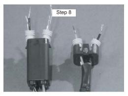
Install a wire seal over each wire so that the unribbed end of the seal is facing the Connector Body and Cap. Check that the wires are aligned properly before proceeding.
