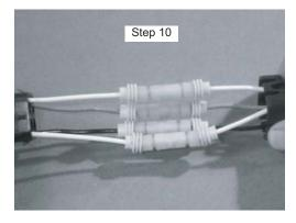
Utilizing "Wire Color Reference Table", begin connecting the wires of the OE Sensor connector harness as described in Step 7. Be sure to avoid criss-crossing the wires. Grasp the wire on each side of the Posi-Lock connector and pull firmly to insure proper assembly.
