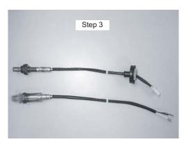
Cut the OE Sensor harness so as to include special clips or grommets. Lay the Bosch Universal Oxygen Sensor beside the OE Sensor and cut the Bosch Universal Oxygen Sensor wiring to the length of the OE Sensor, but do not cut to less than 5" (hex/flange face to end of sensor wire). Proceed to Step 6.
