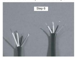
Strip 3/8" of wire insulation from all wire ends. Use proper tools to ensure stripping only the insulation.
