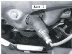
Remove the protective cap from the Bosch Universal Oxygen Sensor and re-install onto vehicle. It is critical to locate wires away from sources of extreme heat and possible abrasion, utilizing any clips or grommets from the OE Sensor wire harness.
