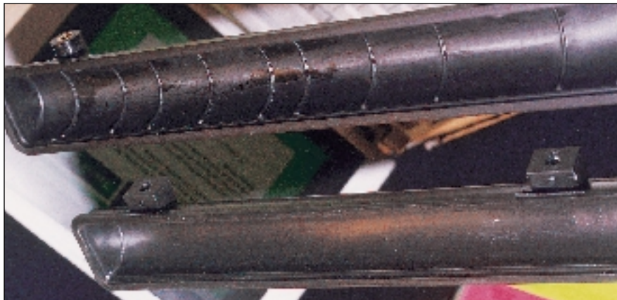
Above: These radiator tanks fit the same core, but the one at the top is an OE-grade design, the one at the bottom a lower-priced aftermarket tank. The OE tank is much shinier, indicating a higher nylon content for greater strength. Right: Close-up of the two tanks shows the OE-grade tank has strengthening ribs inside and a wider support lip around the gasket surface.
