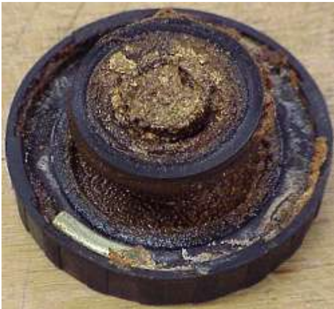
Left: A check with local cooling system shops revealed this cap. It's from a mid-90's Blazer with about 50K miles. Below is the neck.
