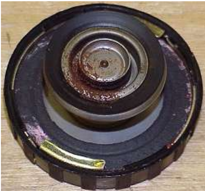
Left: This cap is from a later model Blazer with under 15K miles (notice the onset of corrosion). The cause was not verified, but appears to be iron oxide. If so, the system will need to be chemically flushed.
